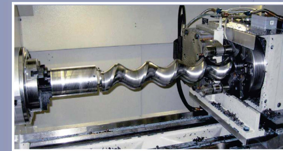
Installation of whirling unit
