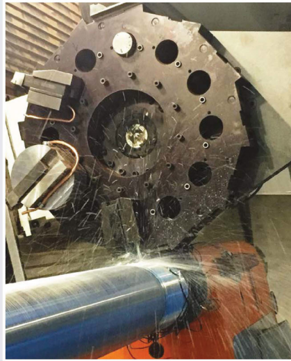
Turret with a special disc with axial and radial toolseats for driven and static tools
