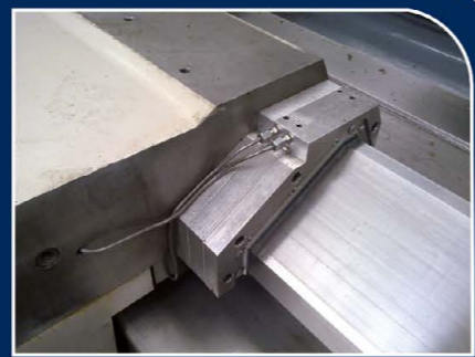
Double scrapers with compressed air for special guide ways security against grinding powder
