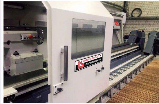
▲ Additional chip conveyor at the front of the machine
