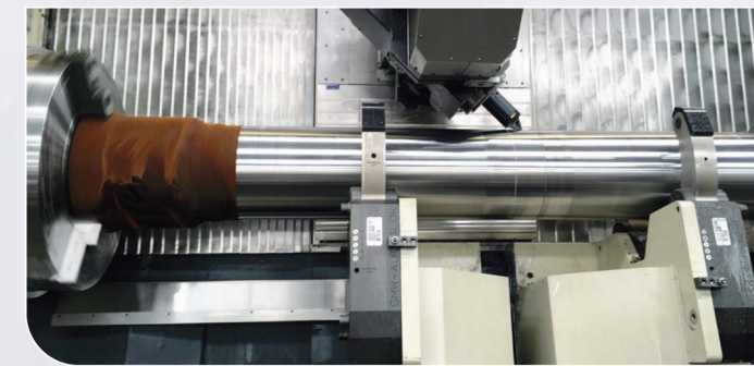
Hydraulic steady rest with independent NC drive
