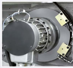
C axis with driven tools: - driven by main motor in combination with hydraulic brake and spindle encoder - full contouring C-axis driven directly by separate servo motor
