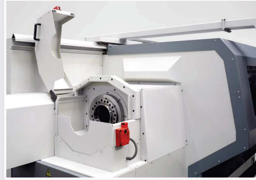
Second spindle nose with complete interlocked covers
