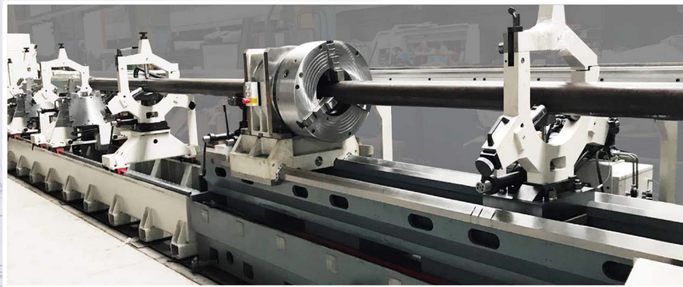
◀ CNC machine with steady rests system for long shafts and pipes
