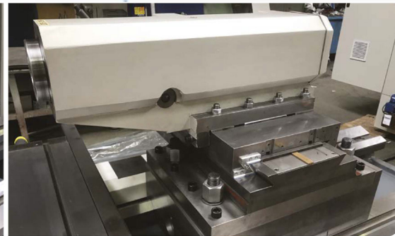
Heavy-duty tailstock with 160 mm (6.3”) quill diameter for increased rigidity and load capacity
