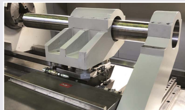
Boring bar holder with quick-change system
