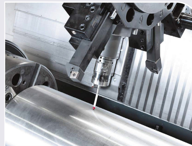
Work piece touch probe installed in turret socket
