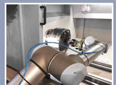
Hydraulic chuck in cooperation with robot
