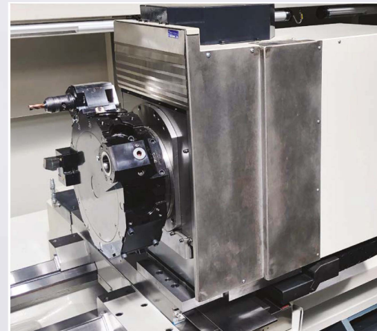
Heavy-duty boring bar attachment mounted on rear T-slots
