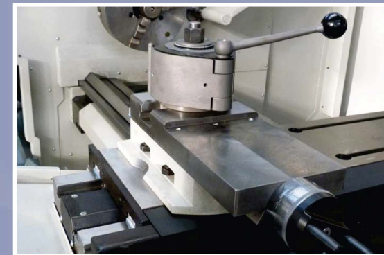
Manual upper cross-slide with Multifix C
