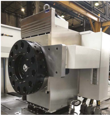
Disc turret with integrated Y-axis
