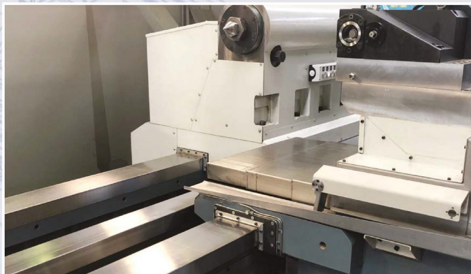
▲ Cross slide without collision with the tailstock
