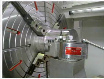
Milling units with automatic Y axis and double spindle, mounted on 4-position head turret
