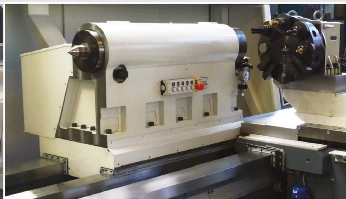
▲ Cross slide without collision with the tailstock
