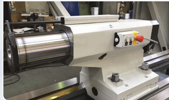
Tailstock with independent drive by push button
