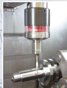
Touch probe for workpiece measuring
