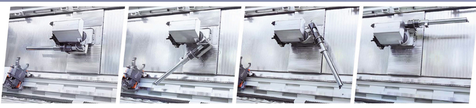
Special boring bar attachment. The unit is designed for boring bar 120 mm (4.7") in diameter. The boring bar is mounted on swivel holder that lets the bar be put on parking position without disassembling.
