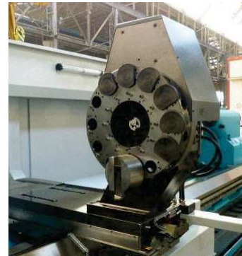
Batuffaldi disc turret for driven tools
