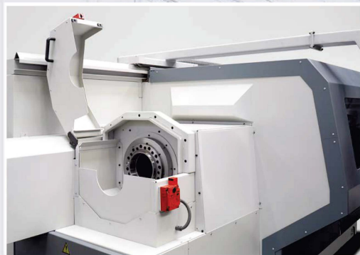
Second spindle nose with complete interlocked covers
