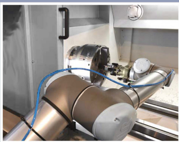
Hydraulic chuck in cooperation with robot
