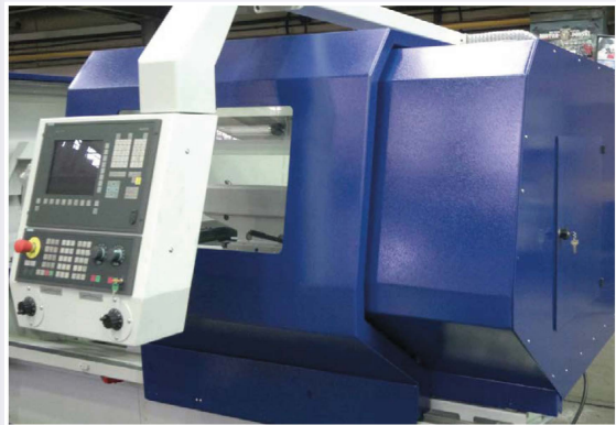
Additional cover of tailstock area
