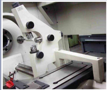
Wide range of self centering hydraulic steady restss
